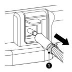
2 Connect the drain hose of the dryer and secure the hose clamp.
