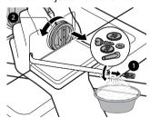
4 After cleaning the drain pump filter, carefully reinsert the filter and screw the drain cap back in clockwise carefully to avoid cross threading and leakage. Reinsert the plug back into the drain tube and place the tube into its holder. **5** Close the cover cap.
