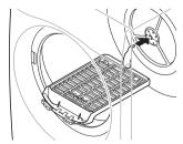
3 Place the dryer rack on the structure above the lint filter and press it to complete assembly.
