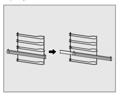
Make sure to slide the tray and wire grill in a correct position as the telescopic runner pins are inserted through the holes on both sides.
