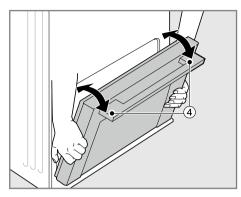
5) Lift and pull the door towards you until the hinge latches are completely loosened.
