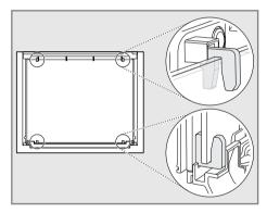
3) Slide in the top glass panel ③ on top of the second glass panel into the oven door.
