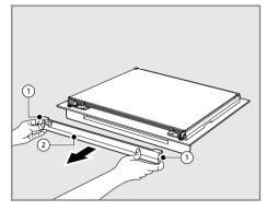
3) With both hands, grab and lift up the glass panel ③ slightly and pull forward to remove it from the oven door.
