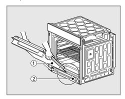
2) Fully insert the hinges ② into the slots ③.
