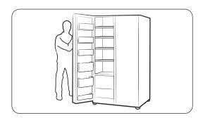
1. Hold the freezer door and hook to the hinge at the bottom of the refrigerator.
