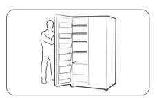
1. Hold the freezer door and hook to the hinge at the bottom of the refrigerator.
