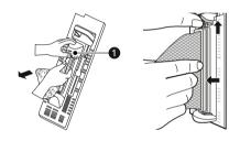
2 Pull the overflow filter forward from the wash tub.
