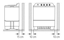
The base openings must not be obstructed by carpeting when the washing machine is installed on a carpeted floor.
