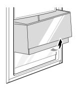
2 Press on the hook inside the top compartment, and then take out the Air Filter.
