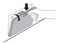
Remove the drain plug from the drain tube first , and then drain the water. Then slowly unscrew the drain pump filter 2 to drain the remaining water and then proceed to remove any debris or objects from the filter.
