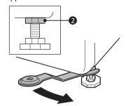
4 Check if all lock nuts at the bottom of the appliance are secured properly.
