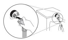
Do not connect the hose to the hot water supply for models with one water inlet. Connect to the cold water supply only.
