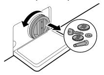
**5** Clean the pump filter and opening with a brush.
