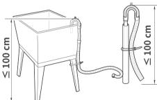
If the drain hose is too long, do not force it back into the appliance. This will cause abnormal noise. • Connect the elbow bracket a within **10 cm** of the end of the drain hose.
