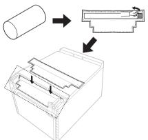
4 Remove the double-sided tape from the lower and front strips.
