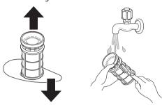
4 To replace the assembled filters, position the spray arm so the wider vee is toward the front. Fit the filters back into the filter holder and secure them by turning the inner filter clockwise until it clicks into place.
